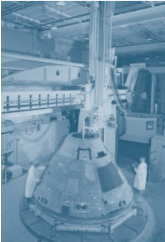
Run by an IBM System/360, a massive turret lathe shapes a heat shield for an Apollo spacecraft.
