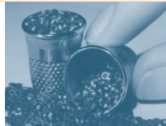
Tiny washer-shaped ferrite cores were the heart of memory technology at the time.
