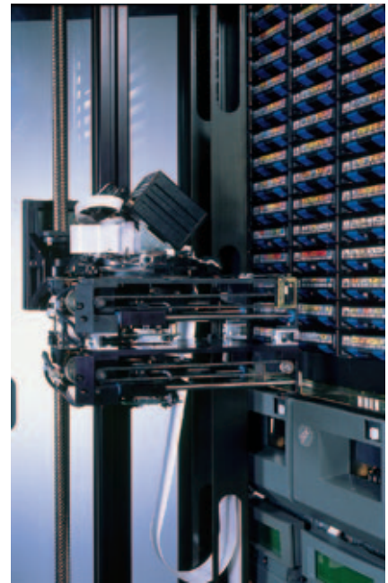
The 3494 cartridge accessor with the dual gripper that provides increased performance and availability.
